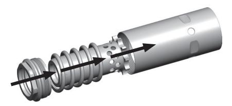
Note: Place a light amount of high quality grease or lube on the inside surface of the Booster Cylinder, O-rings, threaded surfaces, and tapers behind the threads in preparation for assembly.
