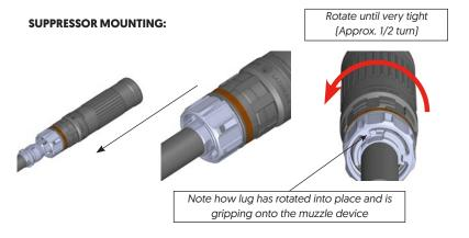
1. With the suppressor oriented to match its TDC marking with the top slot of the muzzle device, slide the suppressor over muzzle device, ensuring it comes to a stop and is resting fully on it.
